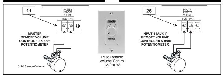
Fig. 21 - Master Remote Volume Control Diagram
